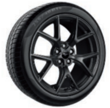
19" 19" x 9.5" front/19" x 10" rear 10 Y-spoke design alloy wheels with high gloss Magnetic painted finish Fitted with 255/40 front and 275/40 rear tyres. (Mach 1 option)
