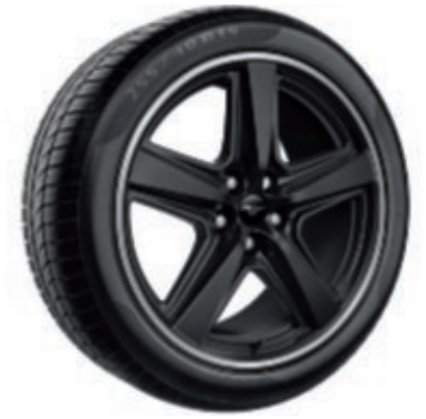
19" 19" x 9.5" front/19" x 10" rear 5-spoke design alloy wheels with low gloss Dark Tarnish painted finish Fitted with 255/40 front and 275/40 rear tyres. (Standard on Mach 1)
